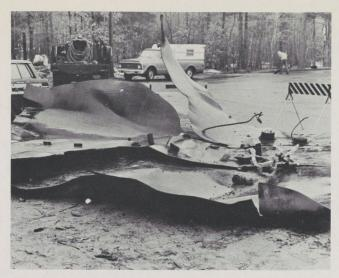
Rear portion of T-24's cargo tank. This has been moved from its original position. (Photos by Lowell Gas Company).
