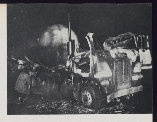
Front portion of T-25 before being moved. The cab was of aluminum and plastic construction. (Photo by Lowell Gas Company).
